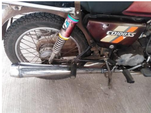
Fig.11. Modified silencer install in bike
