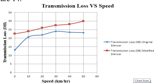
Fig.14. Transmission loss vs speed of original and modified silencer
