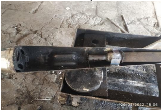
Fig.10. Silencer after cutting the components
