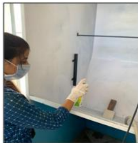
Fig. 3. Liquid paint used for coating the selected raw materials using spray gun.
