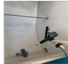
Fig. 4. Powder coating of selected raw materials using the electrostatic gun.
