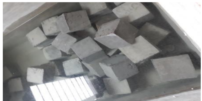
Fig (2.4) Curing of Cubes in Tank
