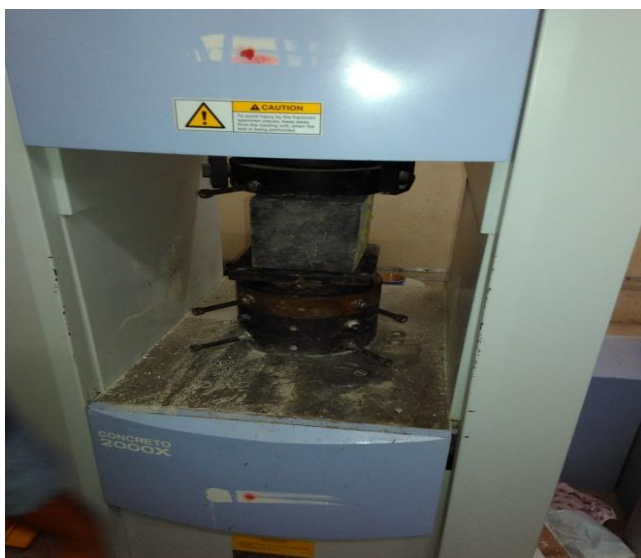
Specimen testing for compressive strength
