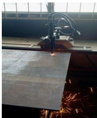
Fig 2: Sectioning of a 10mm thick mild steel plate
