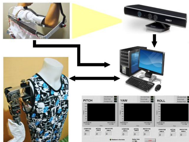
Fig. 6. Process in acquiring data of human shoulder and the robotic shoulder.
