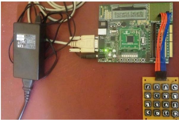
Figure 9. Encryption Output on Explorer 16 Board3
