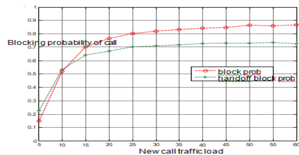
Figure 1.2: simulation result of new Scheme for call admission control with reference to fractal traffic
