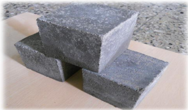
Fig. 2 Cube Specimen for Compressive Strength
