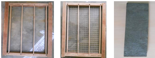
a) Mould for casting flats with glass at the bottom b) Single layer of wire mesh c) Test specimen
