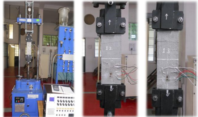
Fig. 3 Tensile Test Set – up with Test Specimens Three ferrocement flat specimens (1-1, 1-2 and 1-3) have been tested with rate of loading as 0.12 mm/min and first crack load and stress – strain relation has been plotted for them.
