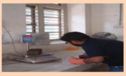
FIGURE 6: DRY WEIGHT OF SAMPLE BRICK
