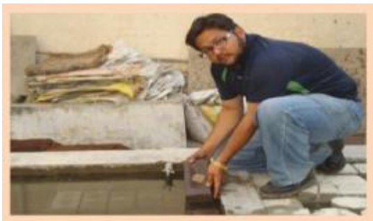
FIGURE 7: CURING OF SAMPLE BRICK
