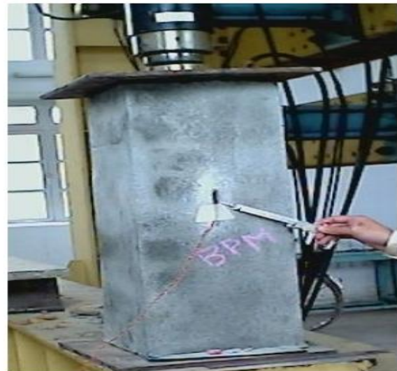
Fig. 2 Plastered specimen with a strain gage at mid-height
