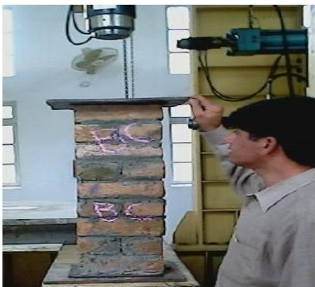
Fig. 1 Plain (unreinforced) brick masonry column
