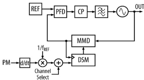
Fig 2-Phase lock loop with delta sigma modulator [5]
