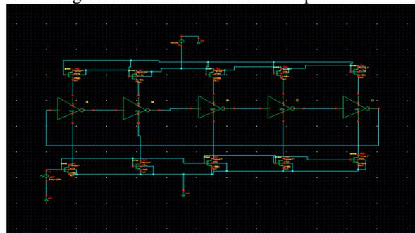
Fig 7 – schematic representation of VCO
