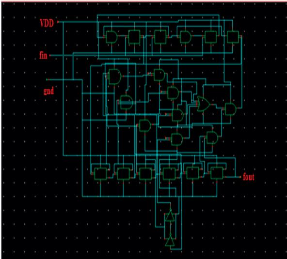
Fig 8 – Schematic representation of MMD.
