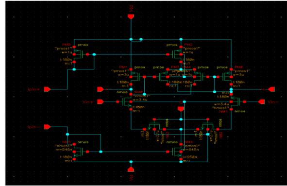
Fig 10 - circuit of the Op amp used in SDM.
