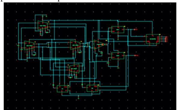
**Fig 21 – Schematic representation of SDM with Filter** Fig 22. shows the transient analysis of the SDM with decimation filter for the time interval of 200ps. The signal net5 of 70GHz is applied to the SDM as input. The signal vout1 is SDM output. The outputs with filters are V1, V2, V3 and V4.
