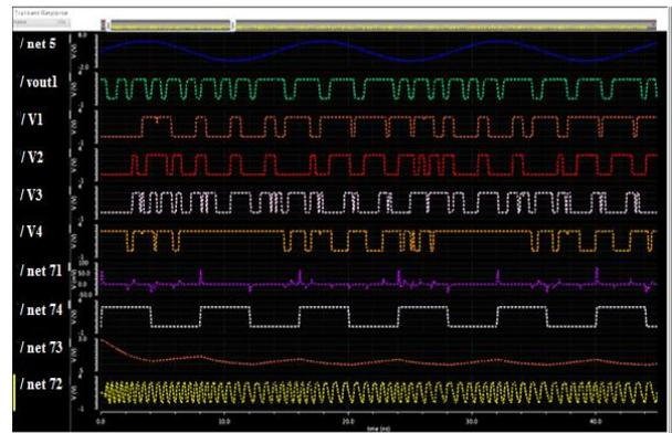
**Fig - 26 Final Output Of combination of PLL and SDM for phase modulation.**
