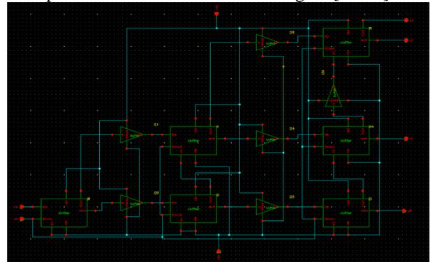
Fig 15 – Schematic representation of third Order CIC Filter
