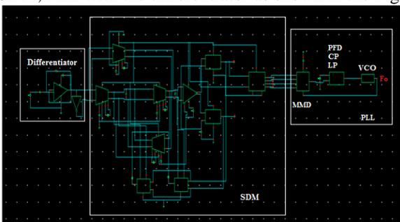
**Fig 25 - Complete Phase modulation circuit for polar transmitters**
