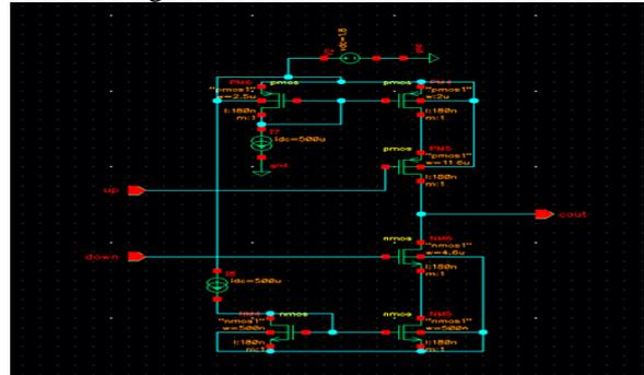
Fig 5 – Schematic representation of the charge pump.
