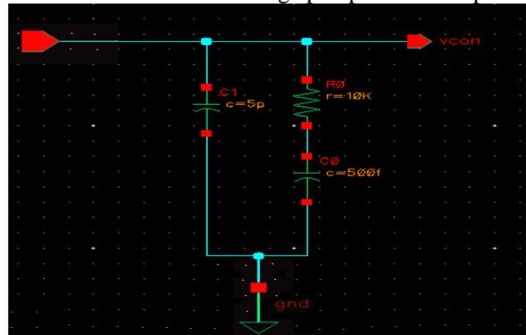
Fig 6 loop filter components.
