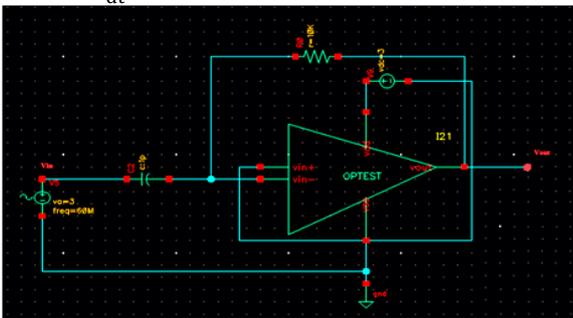
**Fig 17 - Schematic representation of the differentiator.**
