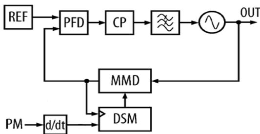
Fig 3- Circuit for the Phase modulation of Polar transmitter.
