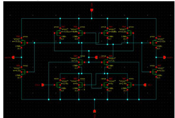
Fig 11- Schematic representation of the CMOS latched-type Comparator.
