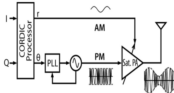
Fig 1 - Conventional Polar transmitters [5]
