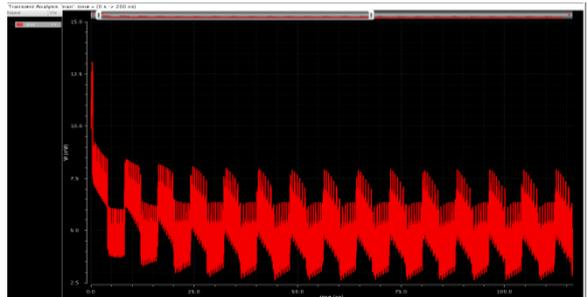
**Fig 20 - Power measurement waveform of complete PLL.** The Fig 20 shows power measurement waveform of complete PLL for a power supply 3V. By using calculator in cadence, the power consumed by complete PLL is 4.277E-3W (4.277mW).
