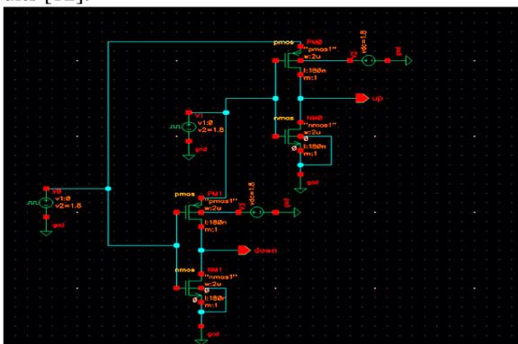
Fig 4- circuit of PFD using GDI cell.
