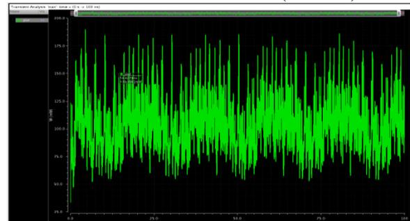
**Fig 27 - Power waveform of Phase modulation of polar transmitter.**
