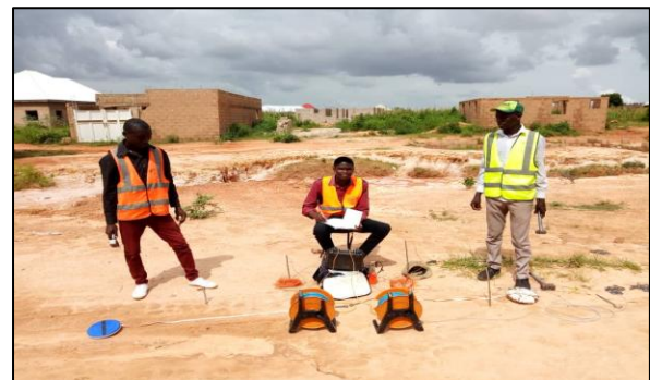
Plate I: Field Setup for VES Data Acquisition (Operators Taking VES Readings Using the Schlumberger Array)
