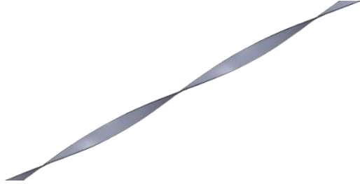
Fig 1. Geometry of conventional twisted tape
