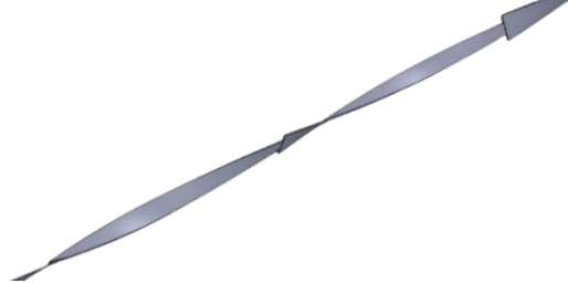
Fig 2. Modified twisted tape without lateral projection
