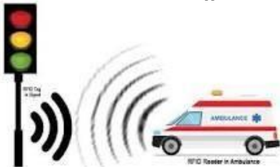
Figure. 5: RFID tag reading Emergency Vehicle
