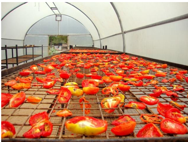
Fig. 11 Drying of tomatoes inside the solar tunnel greenhouse dryer coupled with the biomass heater
