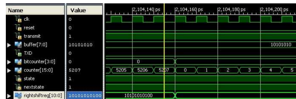
Fig. 10: Simulation result of UART transmitter
