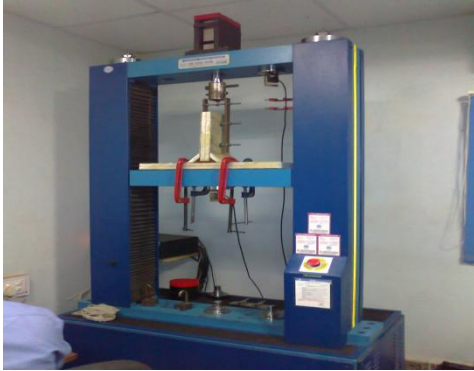
Fig. 11 T-joint loaded to UTM
