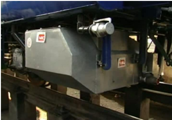
Fig2 : septic tank in Rajdhani express.
