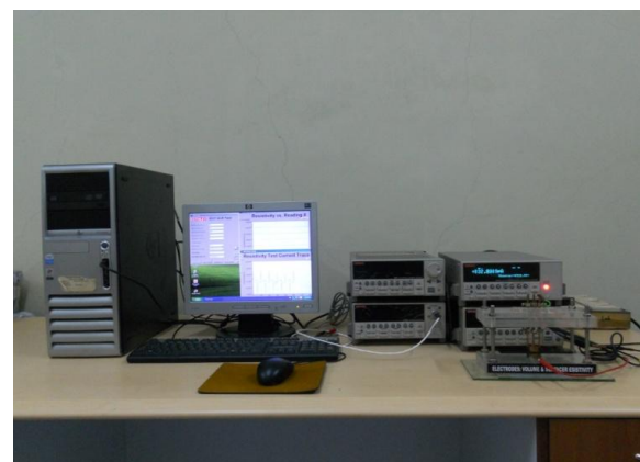
Fig 4. Typical set-up for measurement of DC electrical conductivity of composites.
